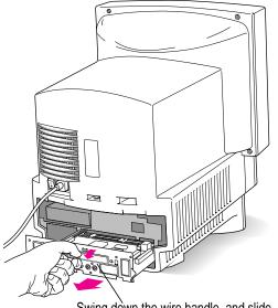
Swing down the wire handle, and slide the logic board out of the computer.
